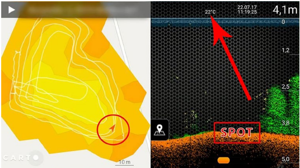
Figure 4.1 — Deeper temperature display
